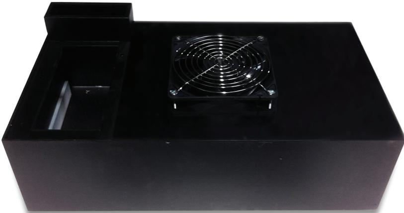
*Hr2 Humidifier with the distilled water deposit*
